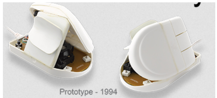
EVOLUENT'S “VERTICALMOUSE” PROTOTYPE. From what I can gather, the first of its kind.
